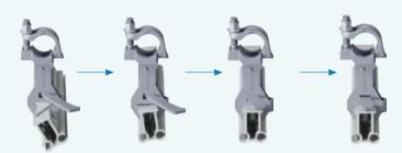
The Keder rail is mounted by means of the Keder rail holder. The Keder rail is positioned by laterally inserting the rail into the fixed part of the holder. By clicking the Keder rail into the end position, the rotatable part of the holder closes automatically and embraces the Keder rail. Keder rail and holder are secured non-positively and positively by a hammer blow on the wedge.
