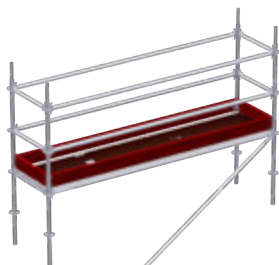
Adding a level (by 2 m per level)
