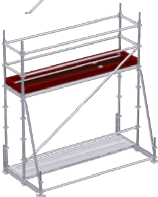
Base structure for adding a level
